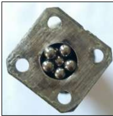
Fig. 2.2 Actual regenerator with porosity 0.6
